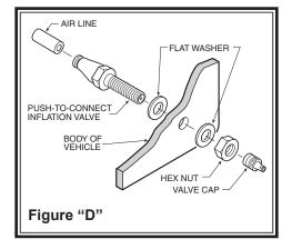
**NOTE:** Too much air pressure in the helper springs will result in stiffer ride, while too little air pressure will allow the air spring to bottom out over rough conditions. Too little air pressure will also not provide the improvement in handling that is possible. **TO PREVENT POSSIBLE DAMAGE MAINTAIN A MINIMUM OF 5 P.S.I. IN THE RIDE-RITE AIR SPRINGS AT ALL TIMES.**
